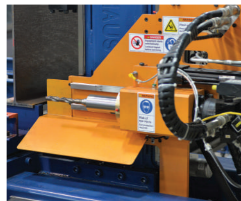
■ ACCURATE LASER DETECTS END OF BEAM
