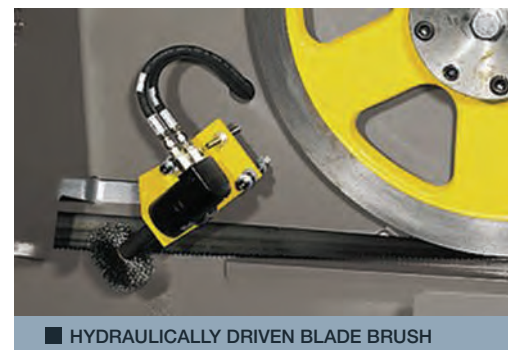
■ HYDRAULICALLY DRIVEN BLADE BRUSH
